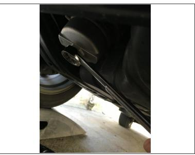
Replace Filter and Drain Plug once all oil has been drained.
