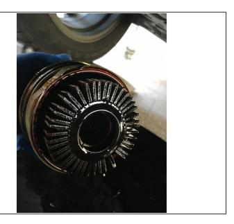
Using a Lexus/Toyota adapter , remove the oil filter housing cap
