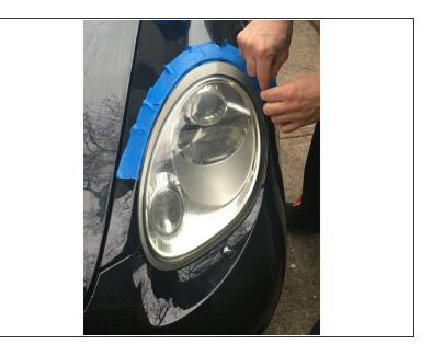
nuse two layers of masking tape to protect to vehicles paint
