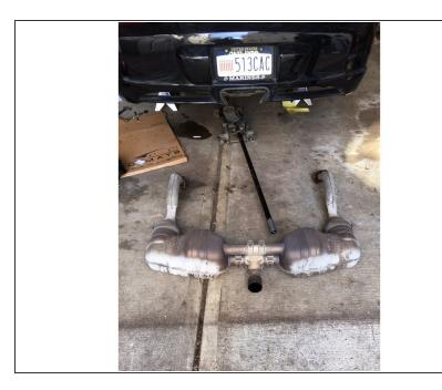
Carefully lift exhaust off exhaust studs and suspension
