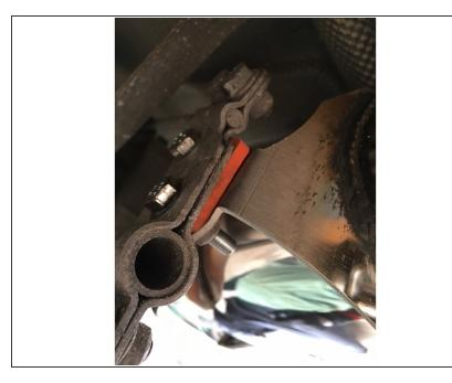
Photo shows Fabspeed supplied rubber gasket
