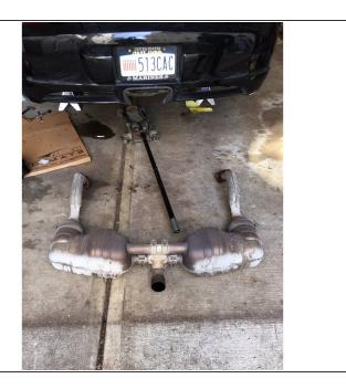
Carefully lift exhaust off exhaust studs and over suspension
