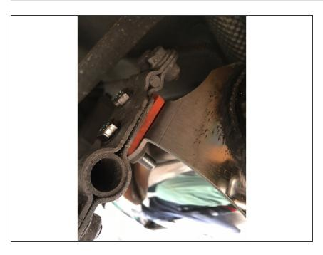
Photo shows Fabspeed supplied rubber gasket
