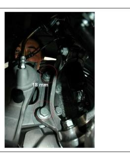
Remove 2 18mm bolt thats hold the caliper. you can remove the caliper and use some zip ties to hang it somewhere.
