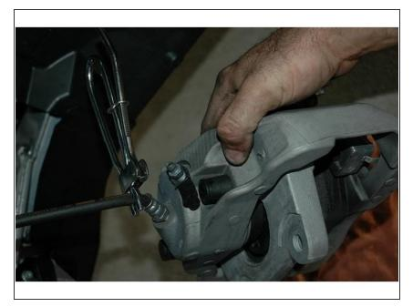
Now pinch the brake line with the pincher.
