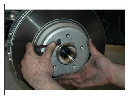
Loosen the 6mm hex on the face of the rotor.
