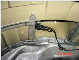
Now, mount the hood switch into the bracket (it basically drops in) and connect the wiring harness to the switch. You must remove the "plug" that is in the connector first. In the pic, the plug is not yet removed.
