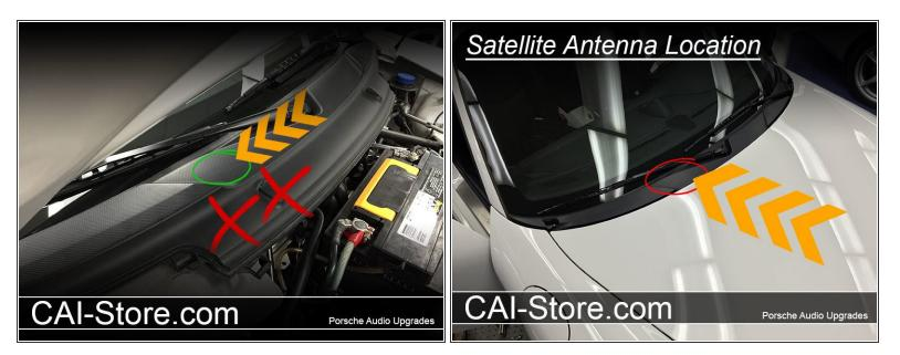
Mount your antenna(s) to the top side of the antenna mount. Make sure that the antenna(s) have a clear view through the plastic that is not obstructed by the metal hood of your vehicle.
