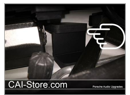
Remove the protective film from the double sided acrylic tape on the bottom side of the mount and stick down in place.
