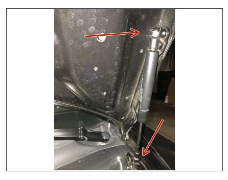
Using a small flat head screw driver, pry open metal clips on the top and bottom of strut
