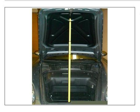
Before removing struts, support the hood. A adjustable painters stick works really well
