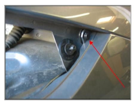
In the far corner is a small fastener securing a tab on the bumper to the quarter panel, remove.
