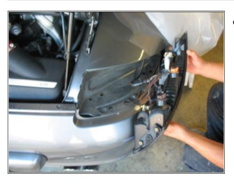
Remove Tail Light and disconnect electrical connections
