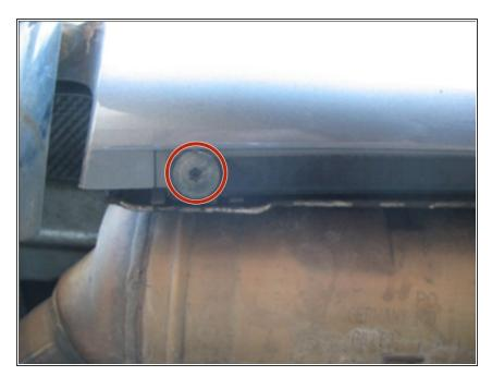
From underneath, by the muffler, remove the 2 bolts holding the bottom center in place.
