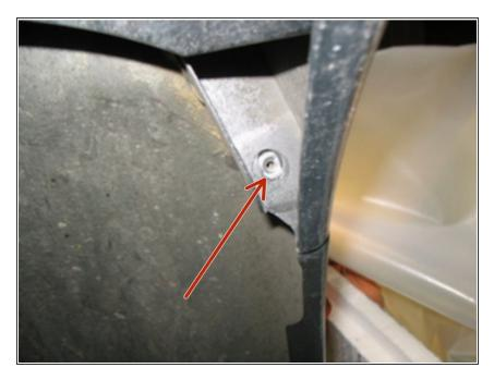
From underneath remove the screw that secures the tip of the bumper to the quarter panel.
