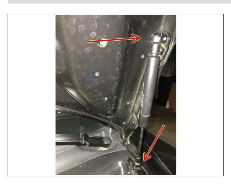
Using a small flat head screw driver, pry open metal clips on the top and bottom of strut
