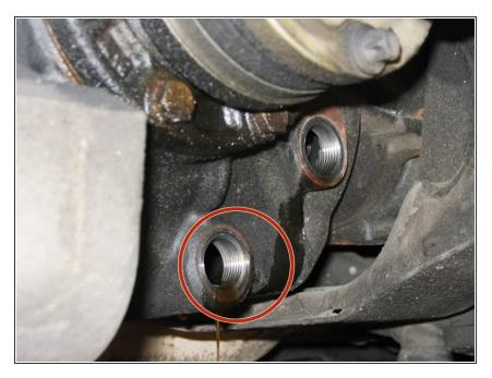
Unbolt drain plug and let it drain for 30 ~ 45 minutes.
