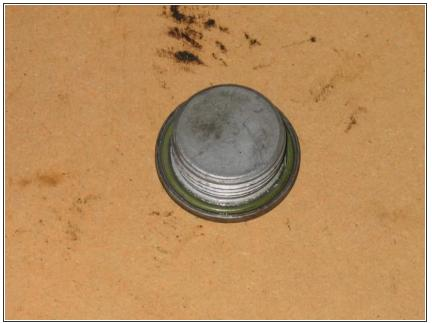
According to Bentley service manual, torque spec for drain/fill bolts are: With O-ring: 60 Nm (44 ftlb) and With sealing washer: 65 Nm (48 ft-lb).
