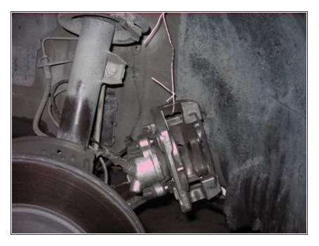
Remove brake caliper and suspend with wire from strut being careful to not bend the brake hose.
