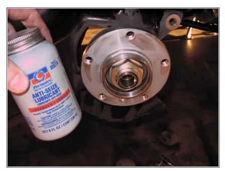
I like to use anti seize on the hub and surround so that brake discs are easy to remove so I lightly coat the hub.
