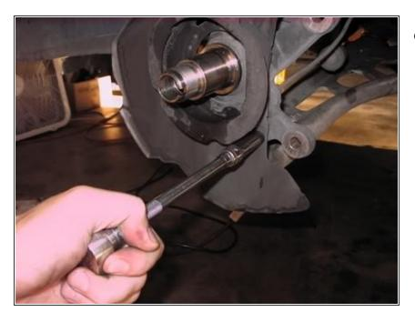
Use a 10mm deep socket to remove the 3 bolts holding the rear brake cover in order to clean it and remove any accumulated junk that might be held in the assembly near the abs sensor and rear seal cover.
