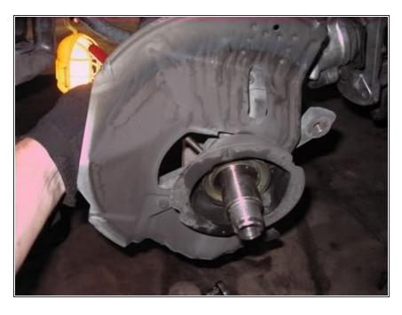
All thats left is the spindle, rear seal cover and brake disc cover so use a punch or something thin to press/gently tap out the inner seal cover to clean it and also the surrounds of the spindle assembly (not required but we all want to do this right).
