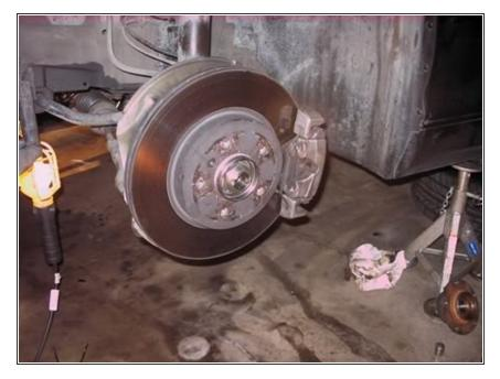
Reinstall the brake disc and torque the retaining bolt to 12 lb ft or per Bentley for your model and then reinstall caliper and torque the caliper to the spindle per Bentley (81 lb ft for my 01 325).
