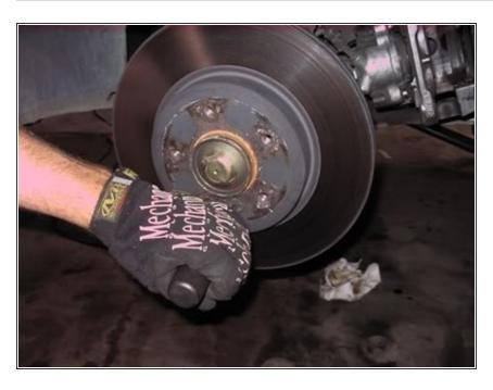
Grab hand impact driver with hex and remove brake disc retaining bolt.
