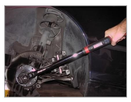
Now you can install and torque the hub nut to specs - check Bentley for your model. Mine was 214 lb ft.
