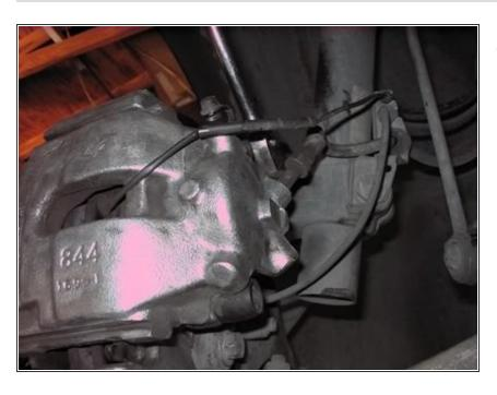
Using 3/8 long ratchet and 16mm short socket remove caliper retaining bolts.
