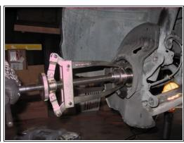
• Use a dremel or long and thin two jaw puller to get off the inner race. I used a two jaw puller so it looked like this.
