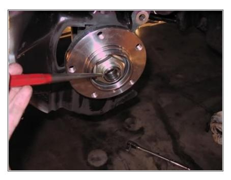
Now using a punch or like dent in the outer portion of the hub nut as a safety precaution.
