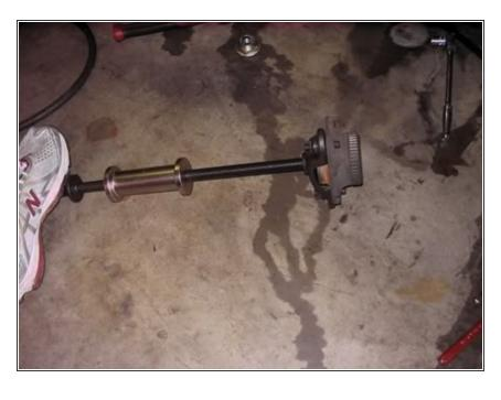
One nice whack with the slide hammer and you should get off the hub and bearing which might just
