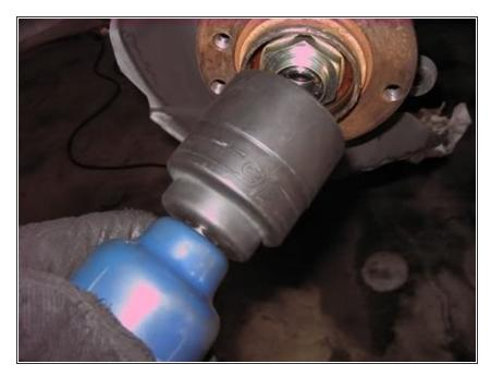
Use 1/2 impact and 46mm socket to remove hub nut - alternatively you could use 18 inch or larger 1/2 ratchet or breaker bar and still easily get this nut off.
