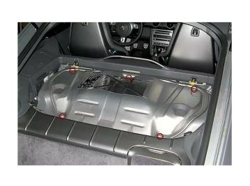
The metallic engine cover is now fully visible. There are 5 screws to remove with the 4 mm Torx driver (red circles).
