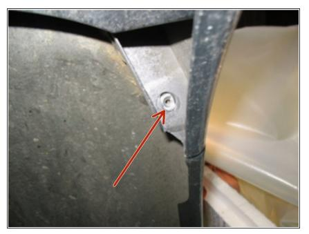
• From underneath remove the screw that secures the tip of the bumper to the quarter panel.
