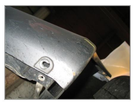
• From underneath remove the 2 screws holding the very bottom edge of the bumper.
