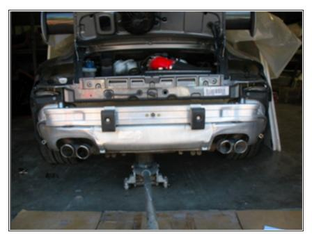
• Carefully slide the rear bumper cover off of the car.
