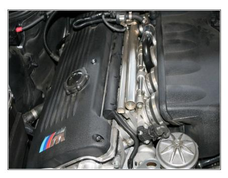
Notice the oil filler cap and the oil filter housing. The filter cap is the large black plastic cap on the left. The metal cylinder is the one with the star pattern top on the lower right.
