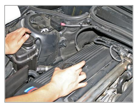
Remove the oil filler cap by unscrewing it counter-clockwise.
