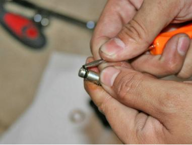
Change the washer at the top of the oil filter housing bolt. Change the rubber O-ring on the oil filter housing cap. Provide the new O-ring a light coating of fresh oil.
