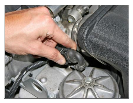
Disconnect the throttle position sensor (simply pinch the clip and pull).
