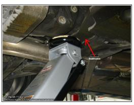
The E46 M3 has four factory jack points (two per side), but you can also jack up the car using these two center points (one in front and one in the rear). Then you can easily place jack stands under the lift pads on the sideskirts/rocker panels.
